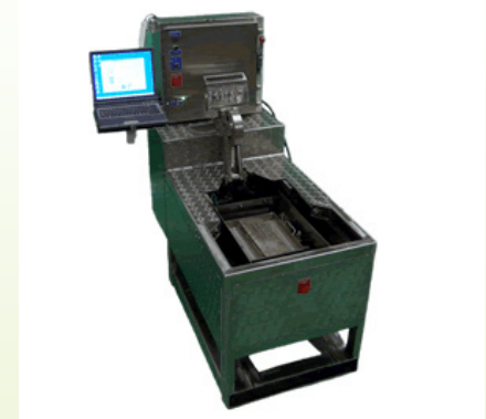
One option for the Hamburg Wheel-Track Test Method is the PMW Single WheelTracker offered by WAPA member Troxler.
