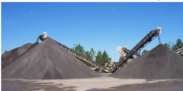
Reclaimed asphalt is an abundant building material—and modern techniques make high RAP levels feasible. (Image courtesy of FHWA)
